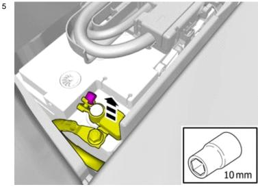
Remove the battery's negative cable.
